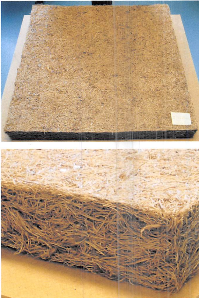
Figure 7. Water glass bonded insulation board made from oil palm empty fruit bunch fibres
