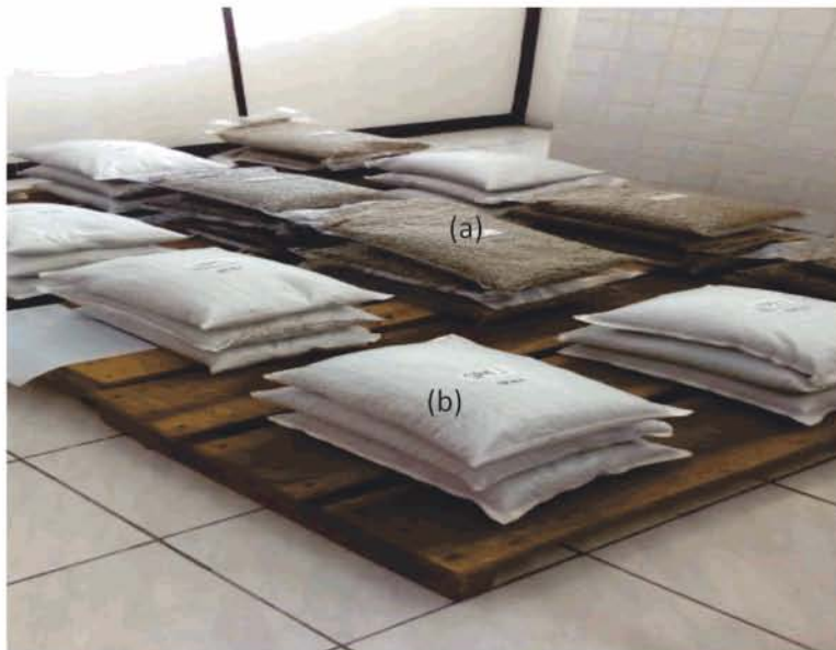
Figure 4 Coffee beans packed in Kantong Semar high gas barrier (a) and polypropylene (b) bags under warehouse conditions
