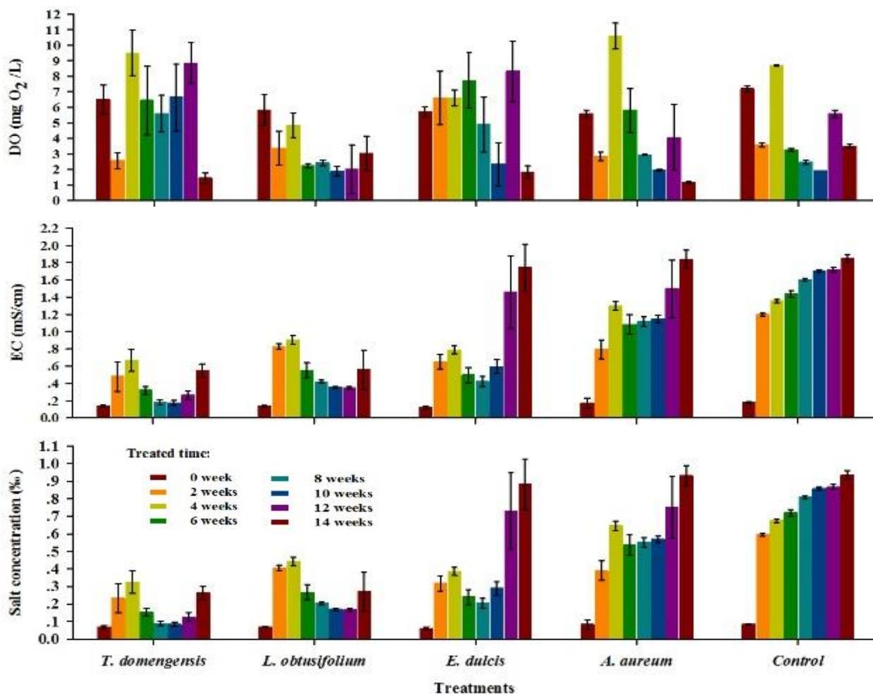
Figure 4 Changes of DO, EC and salt ion contents following the treated time among treatments
