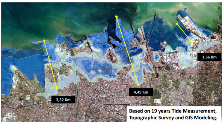
Figure 3. Sea level rise simulation model at Semarang, Central Java Note: Sea level rise = 77.5 cm (100 years SLR simulation model) (Source: Helmi 2021)
